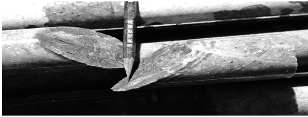
Figure 8. Core from drill hole showing mineralization along a fracture (The pencil pit shows the molybdenum ore).
